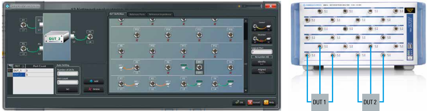
Fig. 5: Measuring multiple DUTs in parallel with the R&S®ZNB T8.
