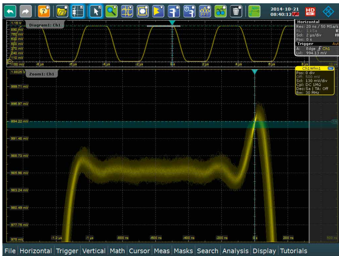
Fig. 5: The high sensitivity of the digital trigger in this example makes it possible to trigger on signal overshoots of less than 9 mV. At a vertical scale of 140 mV/div, this corresponds to only a fraction of one display division.
