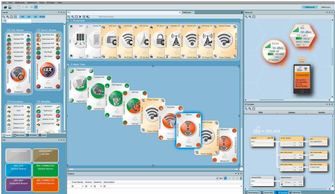
Fig. 5: The R&S®CMWcards graphical user interface for the R&S®CMW500 makes it very easy to compile signaling tests in line with the specification.
