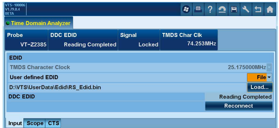
Fig. 7: Menu for configuring the EDID to request a specific output format from an HDMI source.
